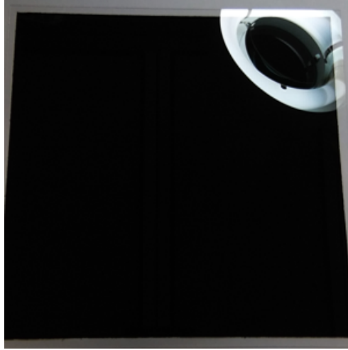
Figure 6.3: 0.3 mm thick float glass plate with an area of 200 \text{ mm} \times 200 \text{ mm} , lined with a \approx 0.1 \text{ mm} thick layer of resistive ink. The ink layer is on the back side of the plate (as evidenced by the reflection of light). To match the area of the aluminium cathode plate, the lined area is only 190 \text{ mm} \times 190 \text{ mm} . The white area in the top-right corner is a reflection of the lamp.
