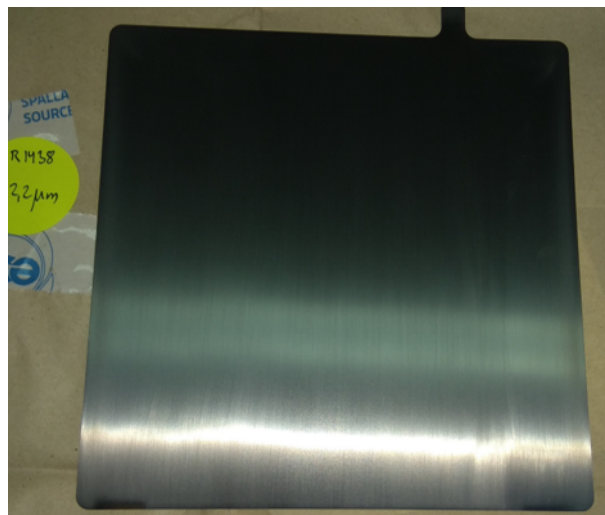
Figure 6.2: 0.3 mm thick aluminium plate (alloy 5754) with an area of 190 mm \times 190 mm, coated with a 2.2 \mu\text{m} thick layer of ^{10}\text{B}_4\text{C} on both sides.
