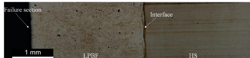
Figure 7. View of failure section in a LPBF/HS sample.
