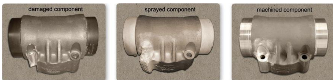
Figure 2.10: Damaged tee box housing from an aircraft flap transmission that was repaired by CSAM and machined in to the “as new” state [Yin et al , 2018].
