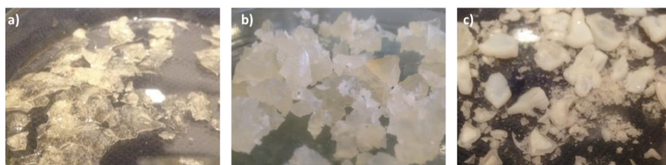
Figure 3.2. Images of CD-HDI at different molar ratio (a) 1:2 (mol:mol); (b) 1:4 (mol:mol); (c) 1:8 (mol:mol).
