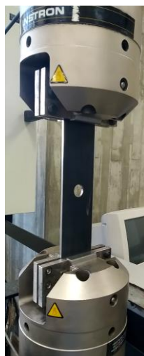
Figure 5.3. Experimental test on S235 bolt hole conducted in a hydraulic machine.
