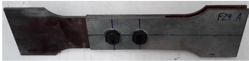
Figure 7.16. Double shear bolted connection.
