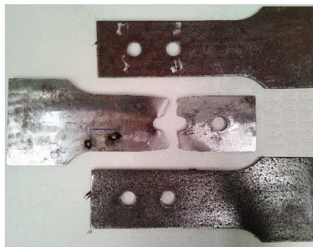
Figure 7.15. Double shear assembly components after test.
