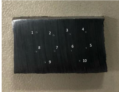
Figure 3.15. S235 sample used in hardness test.
