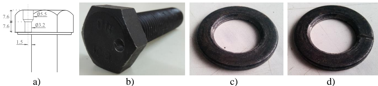
Figure 7.4. a) geometry of injection hole; b) bolt with injection hole; c) chamfered washer to use under the bolt's head; d) chamfered washer to use under the nut with the air scape groove.
