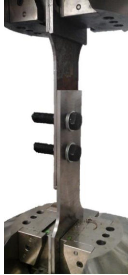
Figure 7.7. Fatigue test on single shear bolted connection.
