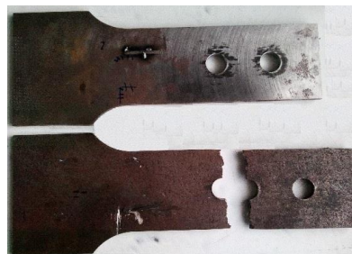
Figure 7.6. Metallic plates from single shear specimen assembly after monotonic test.
