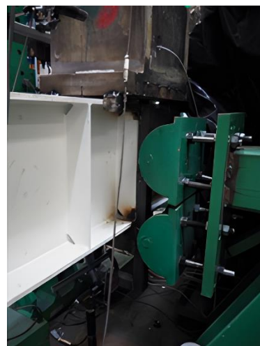
Figure 3.17 – Experimental layout – lateral restraints
