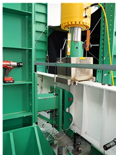
Figure 3.17 – Experimental layout – lateral restraints
