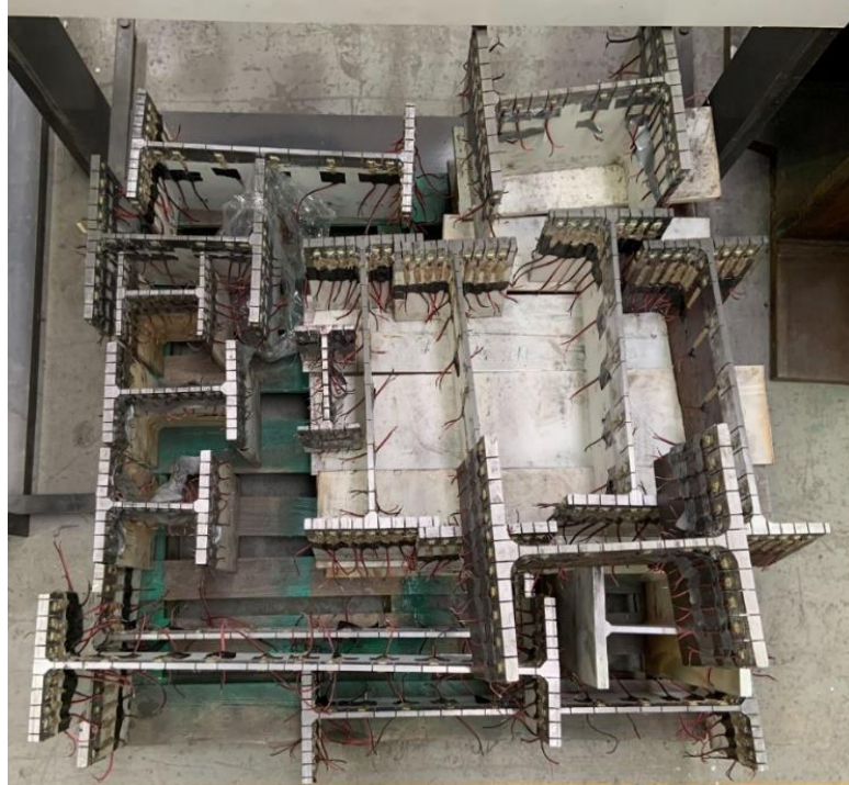
Figure 3.4 – Residual stresses specimens after testing
