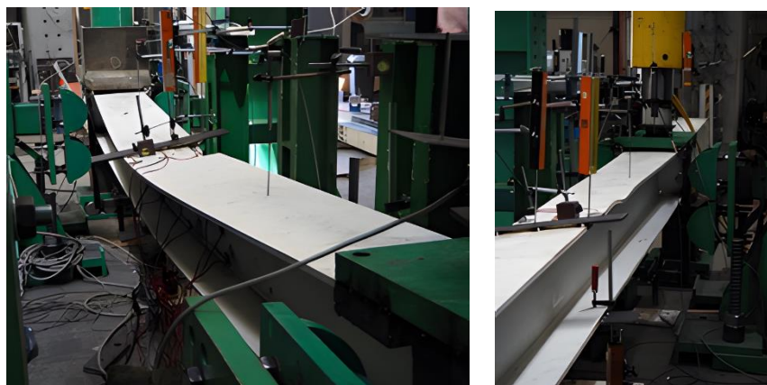
Figure 3.39 - Deformed shape – Tests B4, B5 and B6
