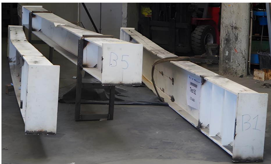
Figure 3.1 – Lateral-torsional buckling specimens after testing
