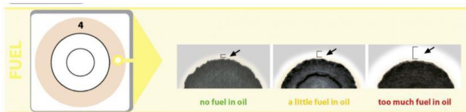
Figure 26 - Fuel Circle Show us if Lubricant is Contaminated by Fuel – Source: (MOTORcheckUP, 2022)
