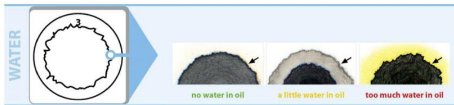
Figure 25 - Jagged Circle Show us if Lubricant is Contaminated by Water or Coolant – Source: (MOTORcheckUP, 2022)
