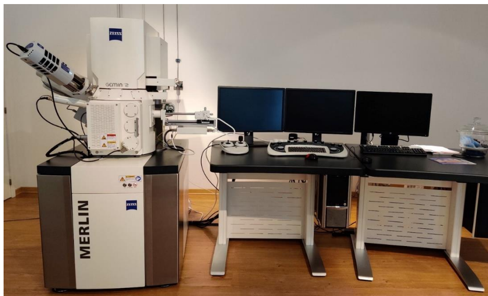
Figure 22. SEM-EDS setup used in this work.
