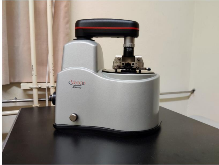
Figure 29. AFM equipment used in this work.
