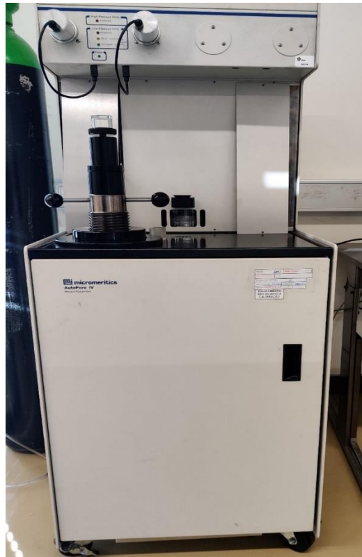
Figure 34. Mercury intrusion porosimeter used in this work.
