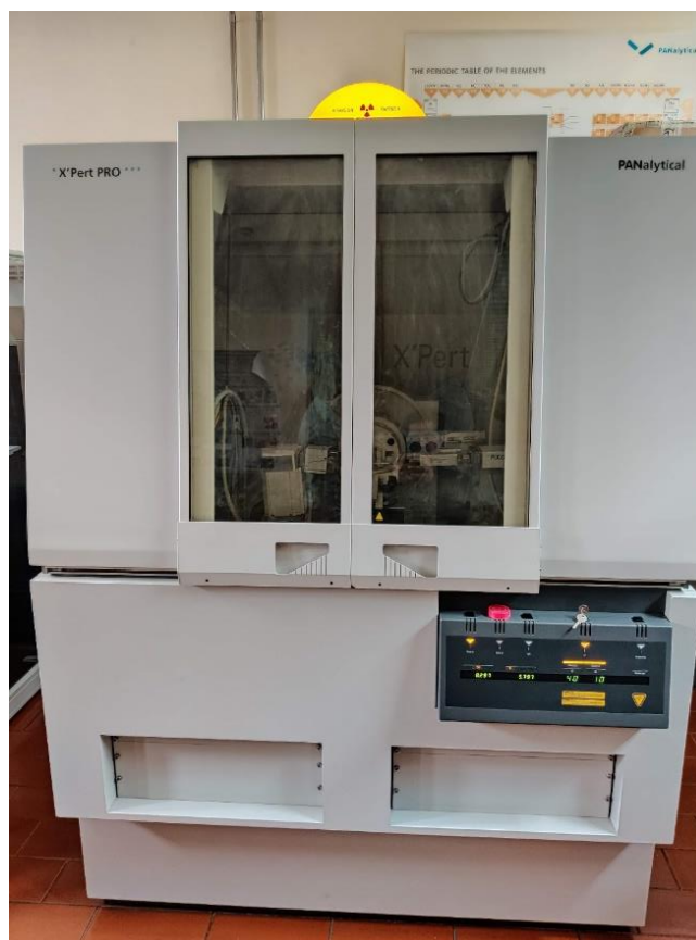
Figure 19. XRD equipment used for structural analysis of the samples.
