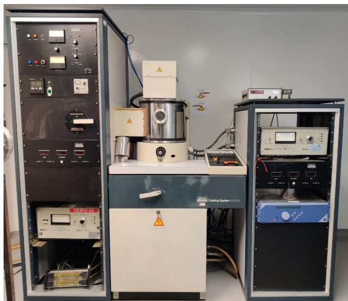
Figure 12. RF magnetron sputtering equipment used in this work.
