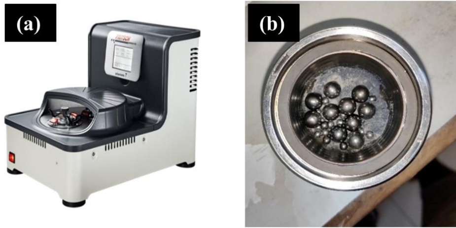
Figure 15. (a) Mechanical equipment used for milling (b) top view of the vial with the powder and balls.
