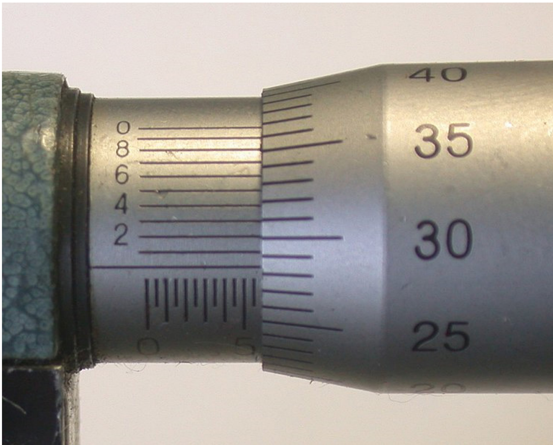
Figure 5.9. A micrometer using the Vernier scale, also known as the nonius scale until the 19 th century (McKechnie, 2019).
