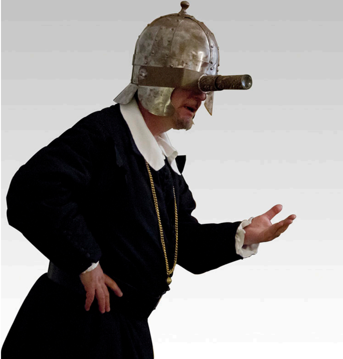
Figure 5.8. A celatone intended for use as a micrometric sky-measuring telescope and worn as part of a helmet. The practicality of this device was defeated by the constant motion of the ship's deck (Celatone (Ricostruzione) IF 102793.Jpg, 2012).
