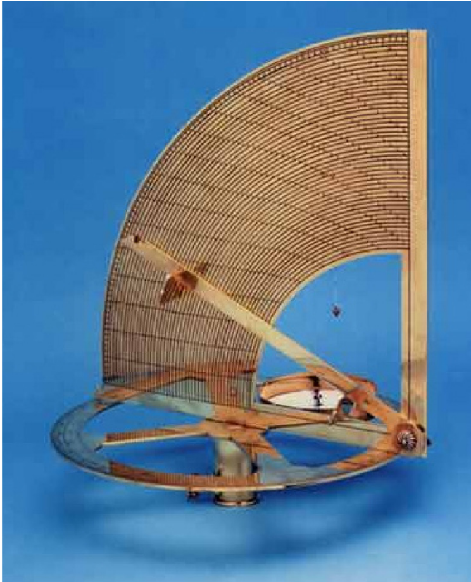
Figure 5.5. Reconstruction of the Kymuyn quadrant with alidade and compass, supervised by Estácio dos Reis and forged by Jorge Leitão from original molds. The reproduction is in the Museu de Marinha, Lisboa (Chance Makes History, n.d.).
