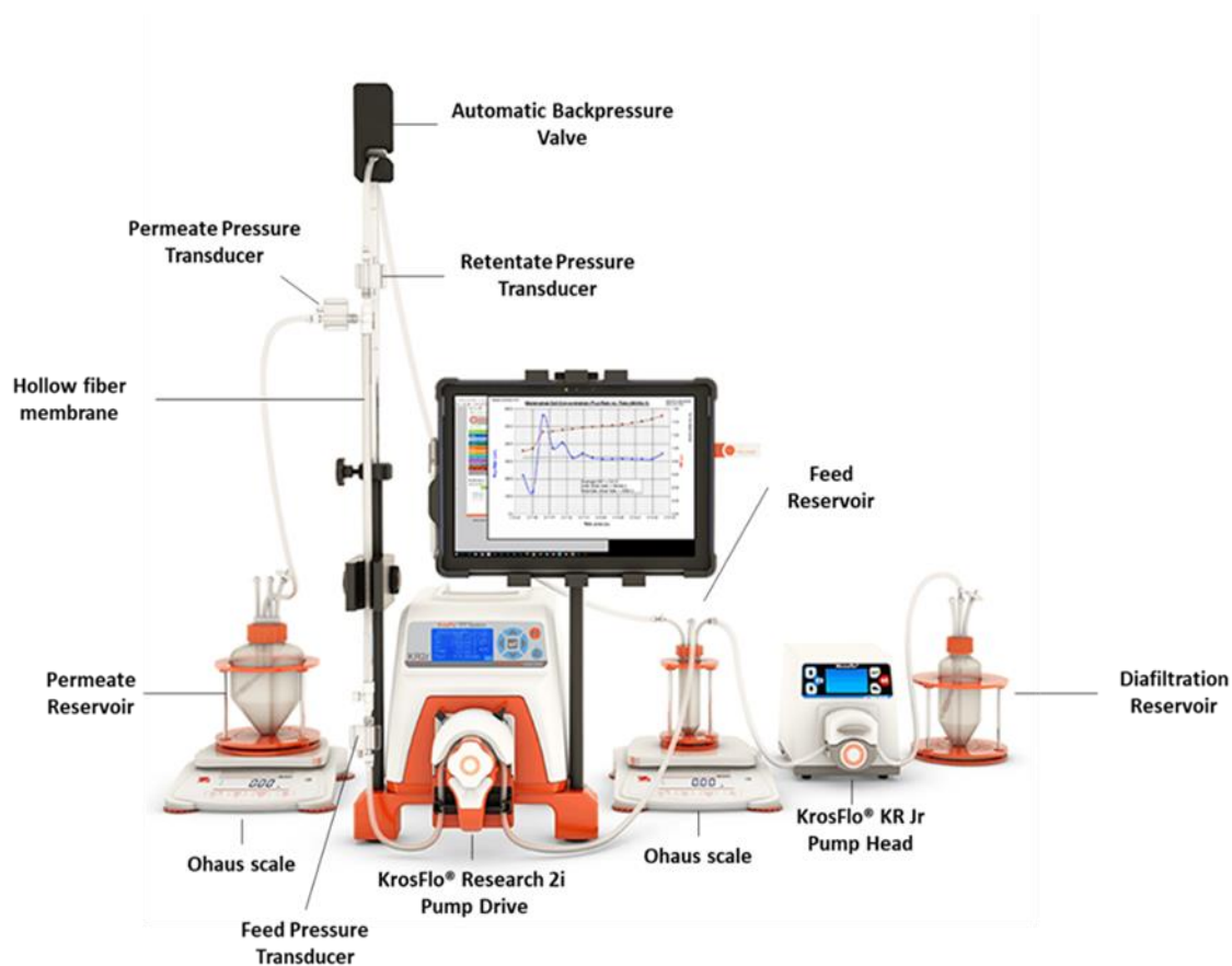
Figure 77. Schematic Representation of KrosFlo® KR2i Tangential Flow Filtration (TFF) System used In-House.
