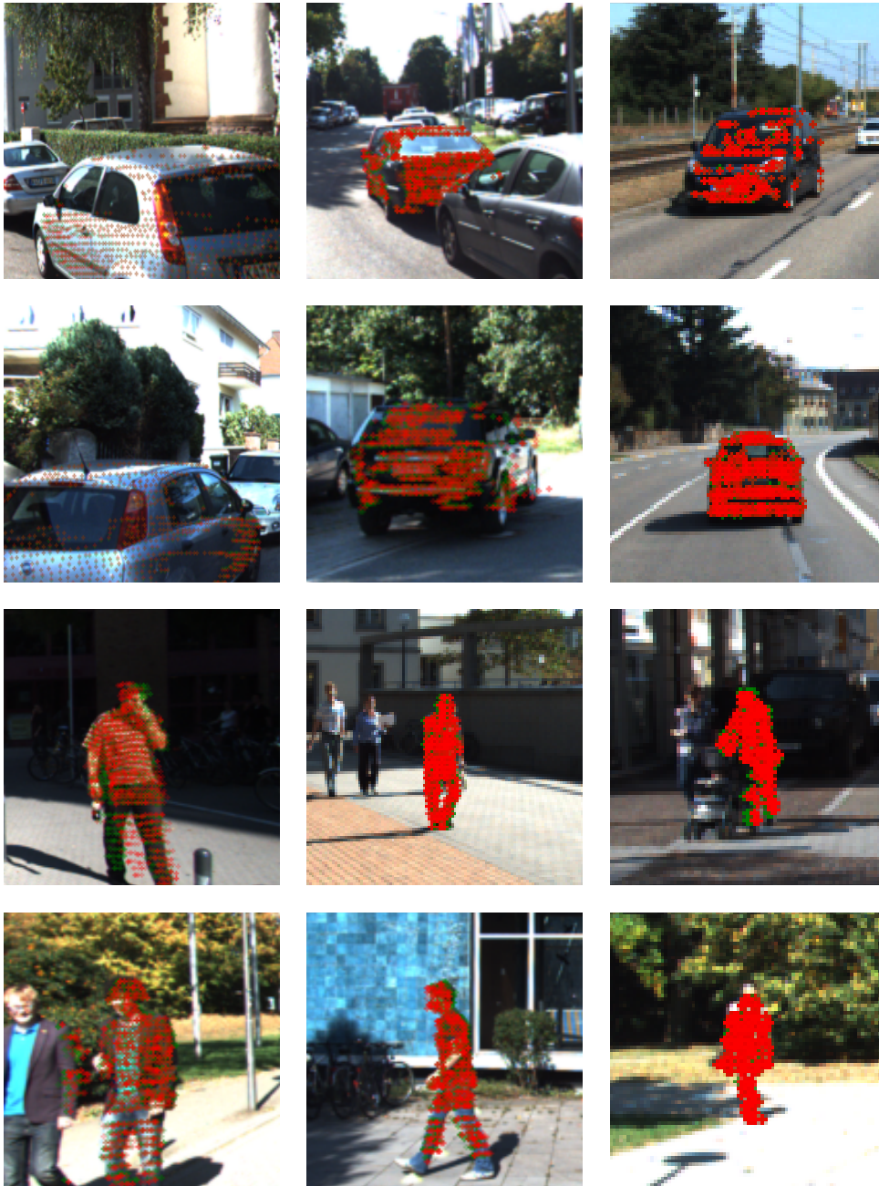
Figure 6.8: Visualization of the method according to the distance on the KITTI dataset, considering only objects with more than 100 points. Green dots indicate the ground truth poses, while red represents estimated poses. Three columns show the results for <7\text{m} , 7\text{-}15\text{m} , 15\text{-}25\text{m} , respectively.
