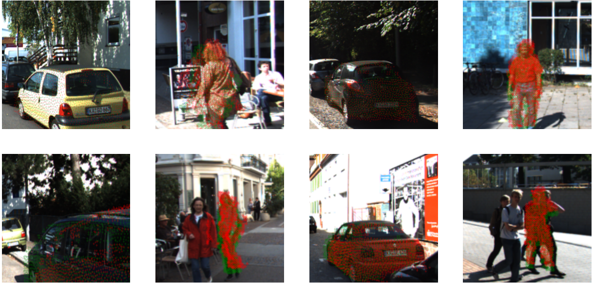
Figure 6.14: Visualization of the DenseFusion: Point Cloud on the KITTI dataset. Green dots indicate the ground truth poses, while red represents estimated poses.
