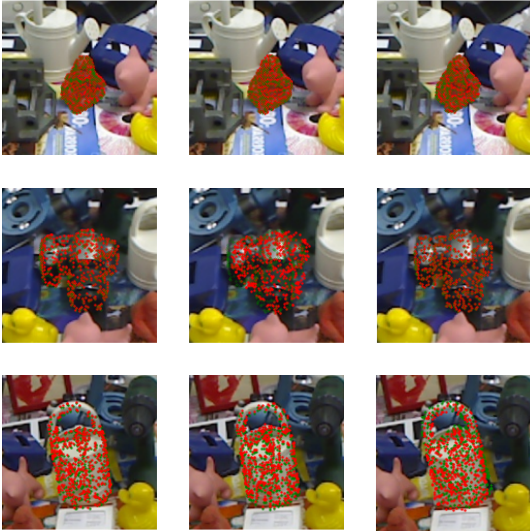
Figure 6.3: Visualization of the multimodal methods on the LINEMOD dataset. Green dots indicate the ground truth poses, while red represents estimated poses. Three columns show the results of DenseFusion, DenseFusion: Depth, and DenseFusion: Point Cloud, respectively.
