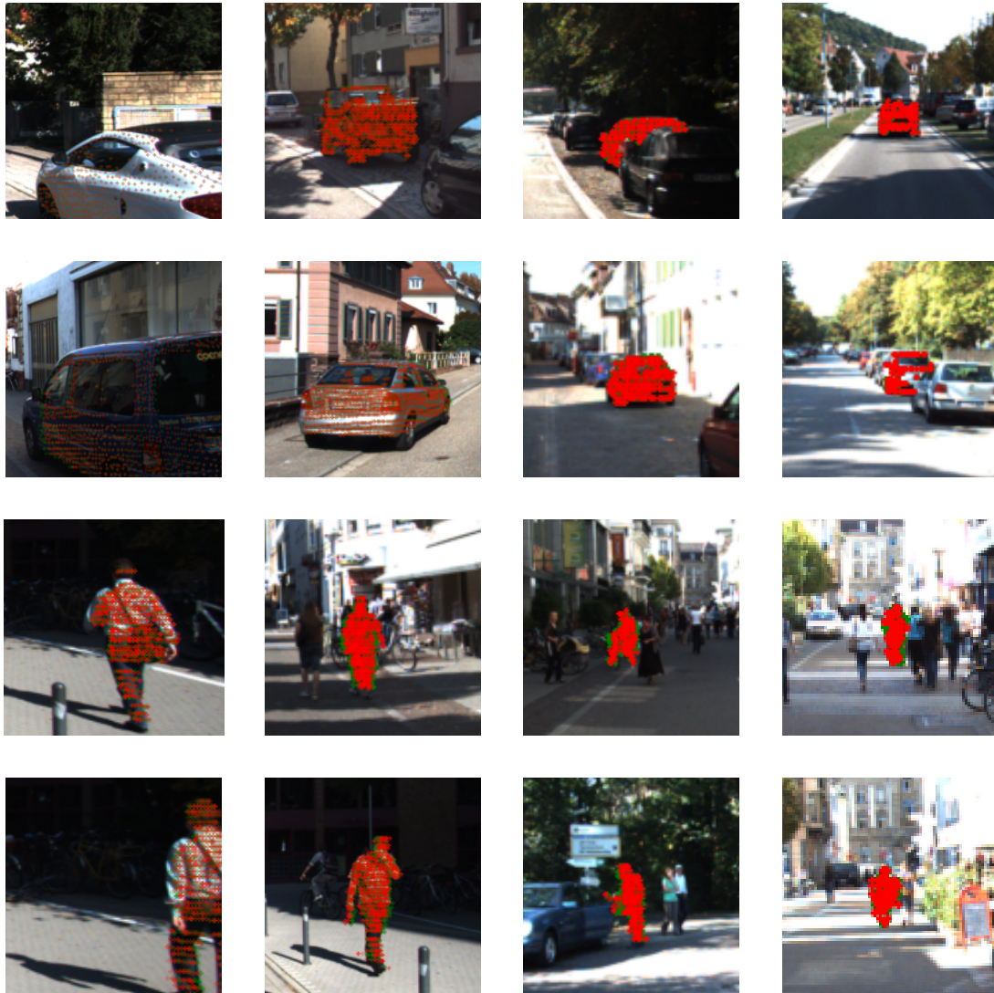
Figure 6.9: Visualization of the method according to the distance on the KITTI dataset, considering only objects with more than 50 points. Green dots indicate the ground truth poses, while red represents estimated poses. Four columns show the results for <7\text{m} , 7\text{-}15\text{m} , 15\text{-}25\text{m} , and 25\text{-}35\text{m} , respectively.
