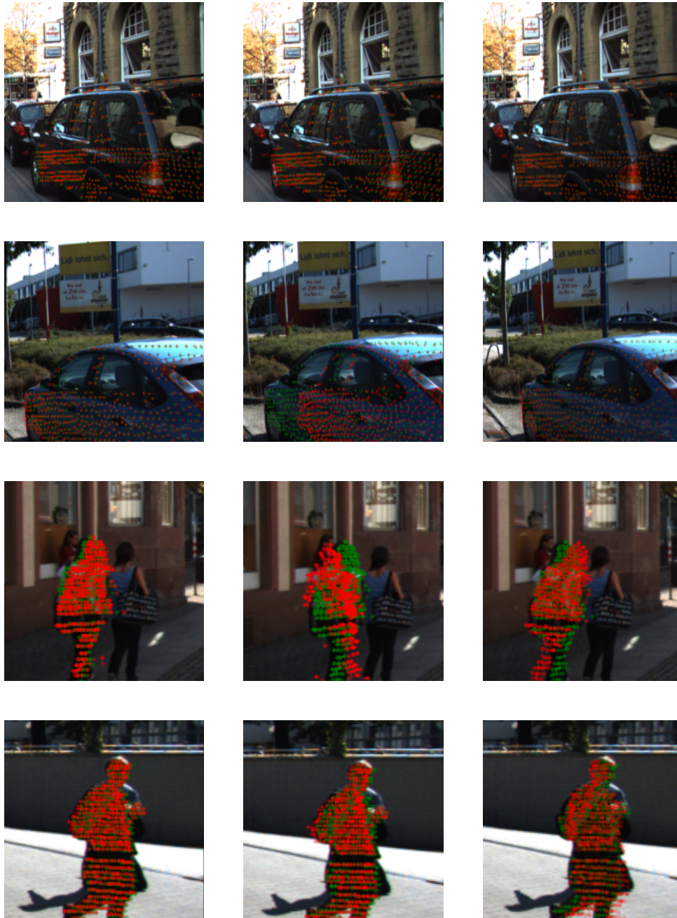
Figure 6.10: Visualization of the multimodal methods on the KITTI dataset. Green dots indicate the ground truth poses, while red represents estimated poses. Three columns show the results of RGB-D, Depth, and Point Cloud, respectively.
