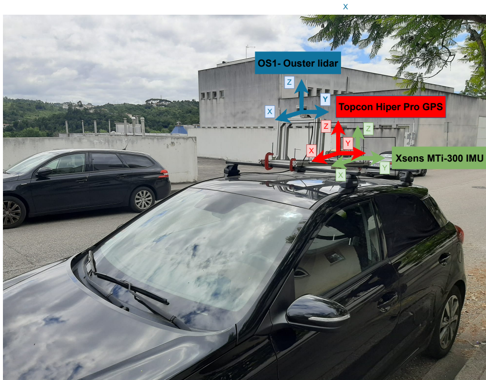
Figure 3.12: System overview. 64-channel Ouster LiDAR installed in the top of the car (sensor in the front row), Xsense MTi-300 IMU installed at the back of the car, and RTK GPS is in between LiDAR and IMU.
