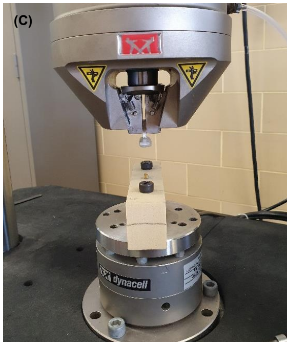
Figure 1: (A) Testing machine. (B) Polyurethane block. (C) Fixed project set: on top, the “T” milled piece with matrix housing of female part, retention device of female part; at the base of the set, the block with implant and Locator® pilar. (D) Milled piece for characterization. (E) On top matrix housing of female part; in the middle nylon inserts of female part; below K-lock and Locator® male part (patrix). (F) Union of the housing to the “T” milled piece by acrylization.
