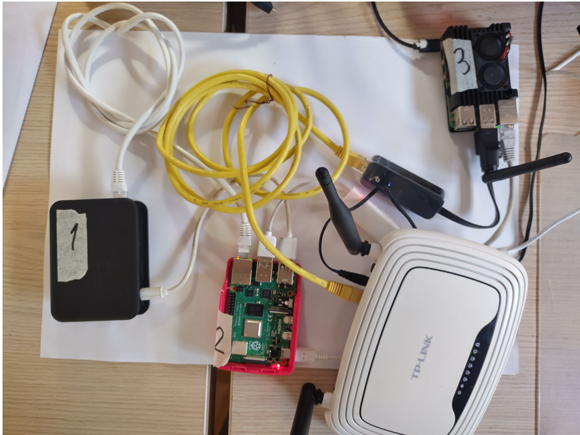
Figure 6.6: INT lab with three P4Pis and one router.
