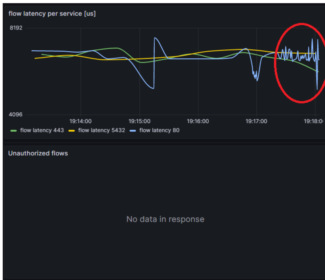
Figure 6.11: Unauthorized access to a SSH service is misreported as an authorized access to HTTP, using an ettercap filter.
