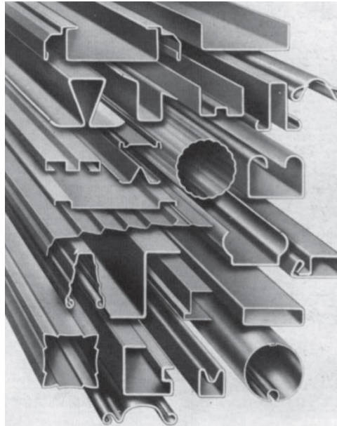
Figure 2 — Common CFS profiles (Wei-Wen et al., 2020)
