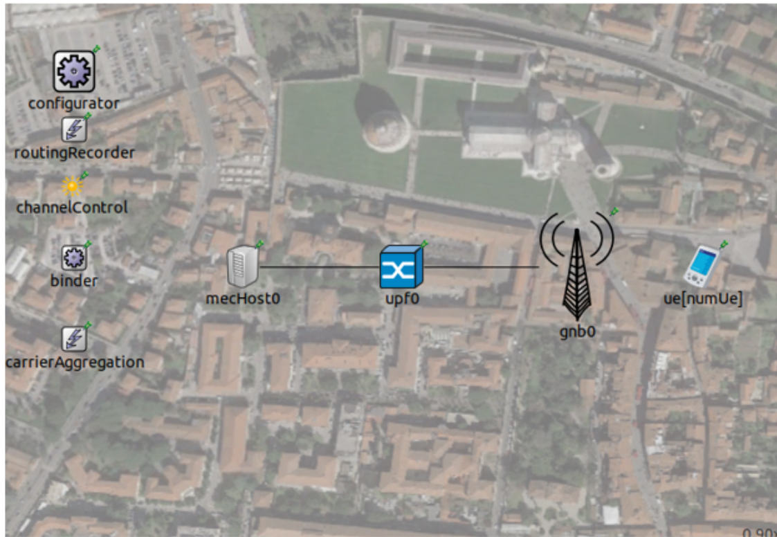
Figure 5.3: SIMU5G Network Topology [12]
