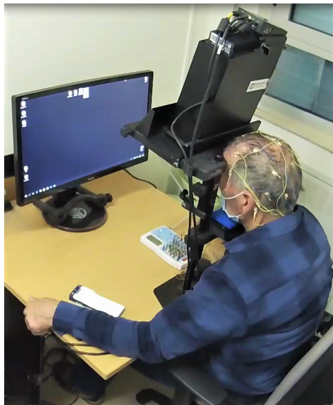
Figure 3.3: Participant with EEG and Percept TM PC performing the eye movements tasks in the EyeLink1000Plus.
