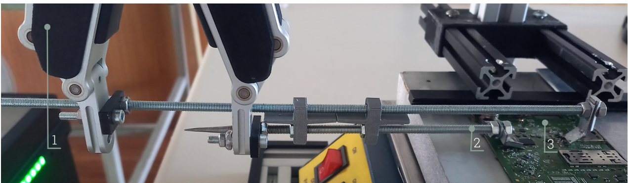
Figure 4.3: Prototype 2 of the tool fabricated to remove PCB's components. (1) gripper, (2) tool, and (3) mobile phone's PCB.
