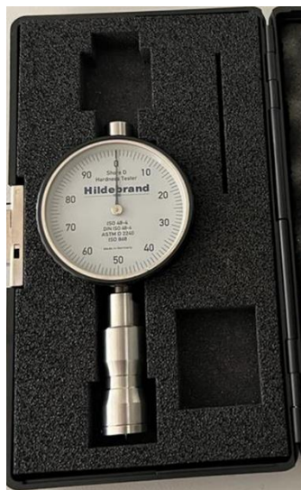
Figure 19. Shore (Durometer) Hardness Tester used in this work.
