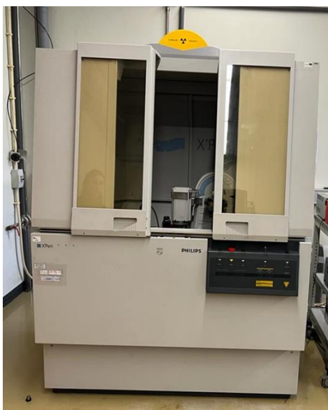
Figure 17. Philips XPert XRD equipment used in this work.
