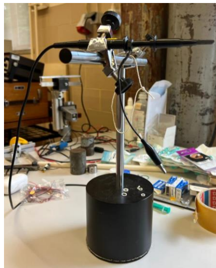
Figure 20. Dynamic Young's modulus measurement apparatus.
