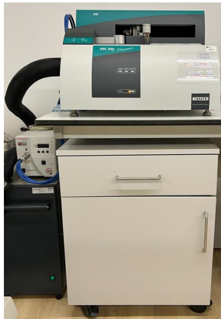
Figure 18. DSC equipment (NETZSCH-DSC 204 f1 phoenix) used in this work.
