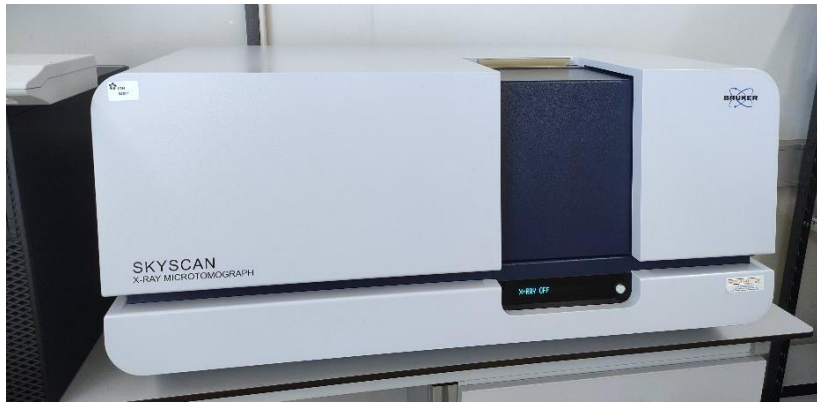
Figure 15. SKYSCAN X-ray microtomography equipment used in this work.
