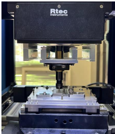
Figure 21. Pin on disk tribometer (Rtec).
