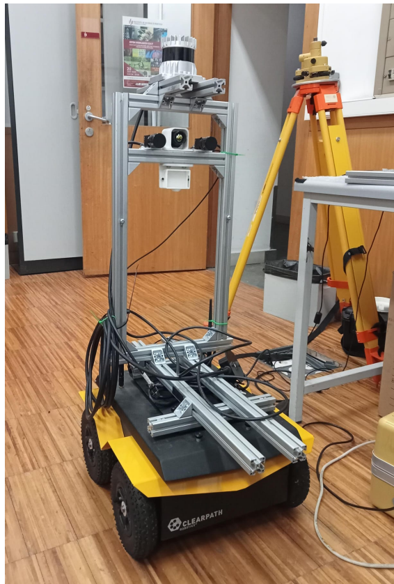
Figure 3.2: Mobile robot created and used to capture and collect the images inside the department DEEC-UC.
