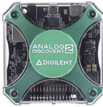
Figure 3.8: Image of the Analog Discovery 2 - Digilent [42].
