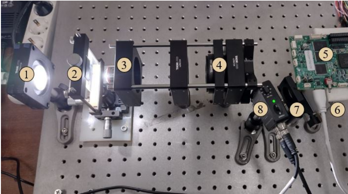
Figure 4.16: Experimental-set up [6]. 1- Light Source; 2- Target; 3- Objective lens; 4- Tube lens; 5- DLP; 6- Sandblasted glass; 7- Positive lens; 8- Photodiode.
