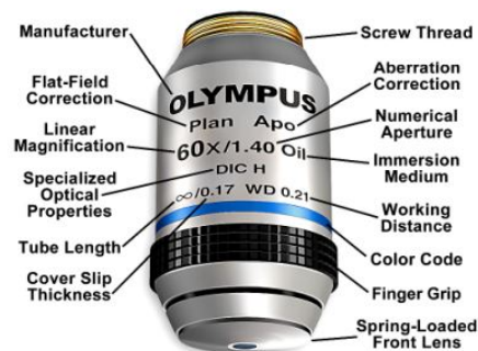
Figure 2.4: Specifications of a microscope objective lens [22].
