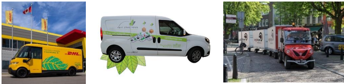
Figure 35 – Examples of electric vehicles used in last-mile delivery: electrical truck, electrical van, and solar-powered electric mini-train (adapted from (Benelux, 2023), (Vous, 2023), and Teubner, 2013), respectively).
