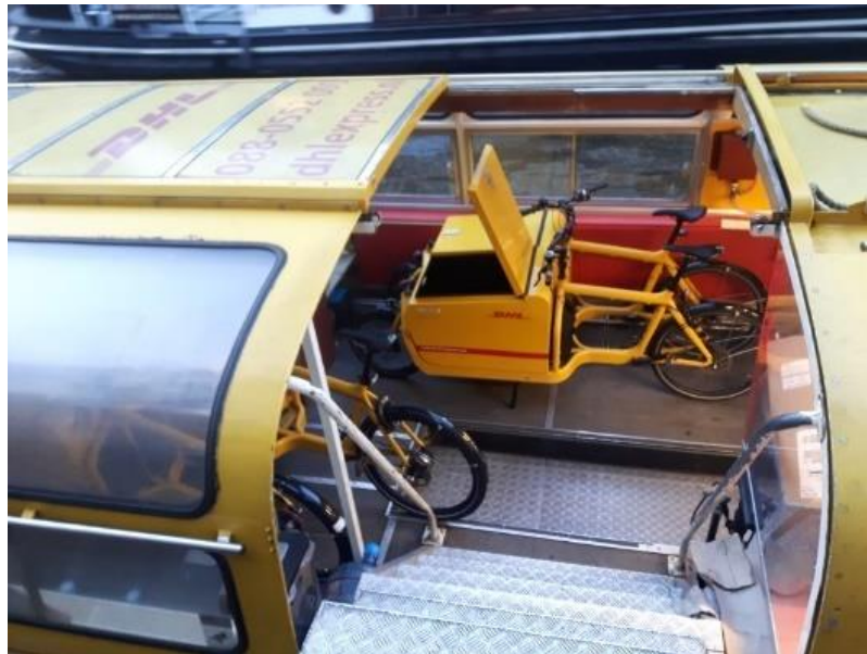
Figure 33 - DHL's Conventional Bikes on a Floating Distribution Center for Last Mile Delivery Source: (Kuzeyliden, 2023).
