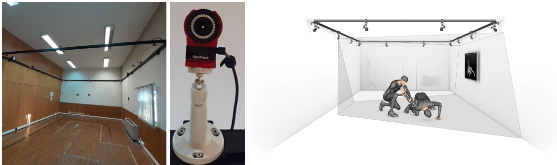
Figure 3.8: The ISR optical motion capture room layout with ten cameras that emit IR rays reflected on the MoCap suit with the passive markers to module the motion.
