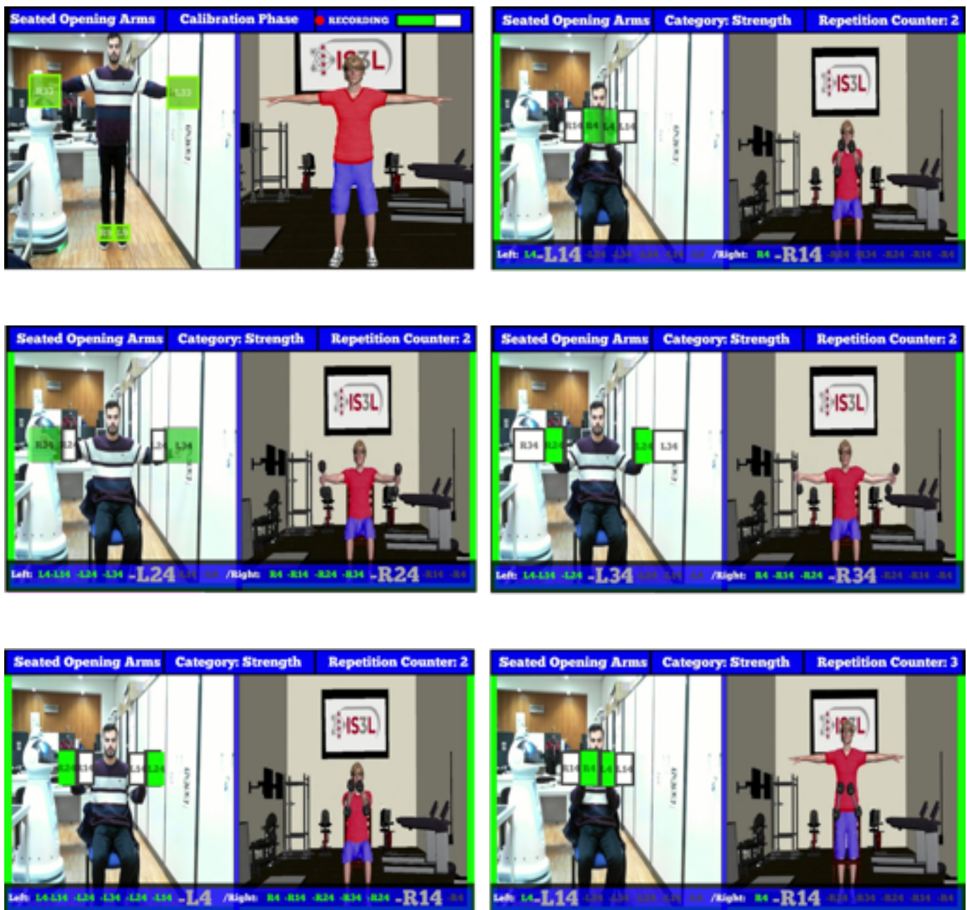
Figure 5.19: Sequence of Events when performing a Seated Opening Arms Repetition, where the coach is waiting until the user reaches the critical points of the exercise.
