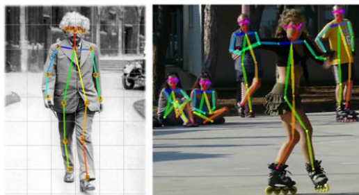
Figure 4.1: Pose Estimation using each of the approaches mentioned above, where on the left side is the single-person and on the right side the multi-person approach.
