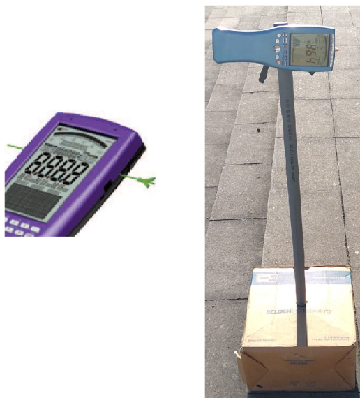
Figure 3.4: NF-5020 single axis E-field sensor and External survey for Vertical E-fields[17].
