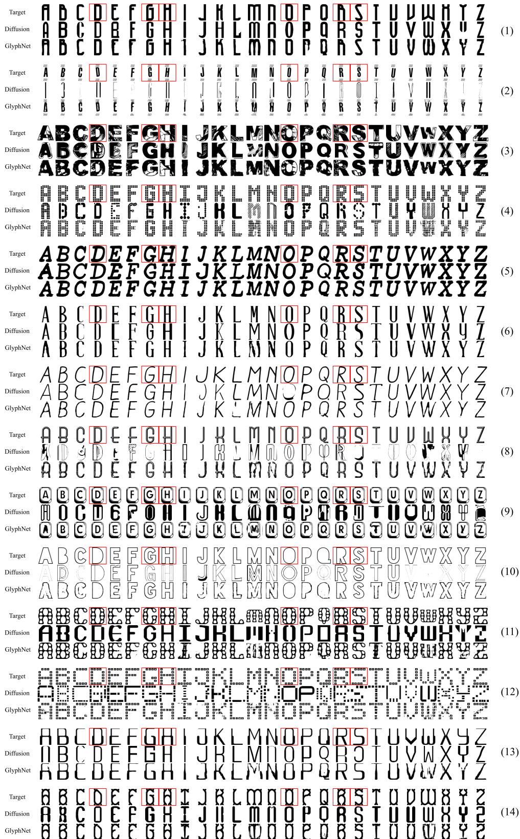
Figure 4.10: Comparison of outputs produced by the diffusion model and GlyphNet given the subset (D,G,H,O,S,R) as input for test samples. Each row is composed of the target font at the top with inputs annotated in red, followed by the generated outputs.
