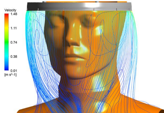
Figure 1.4: Air curtain streamlines. Adapted from [31].
