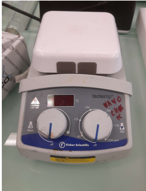
Figure 5.3: Heat Plate Stirrer of Fisherbrand Isotemp in Ceramic used to the Heat Soaking treatment.
