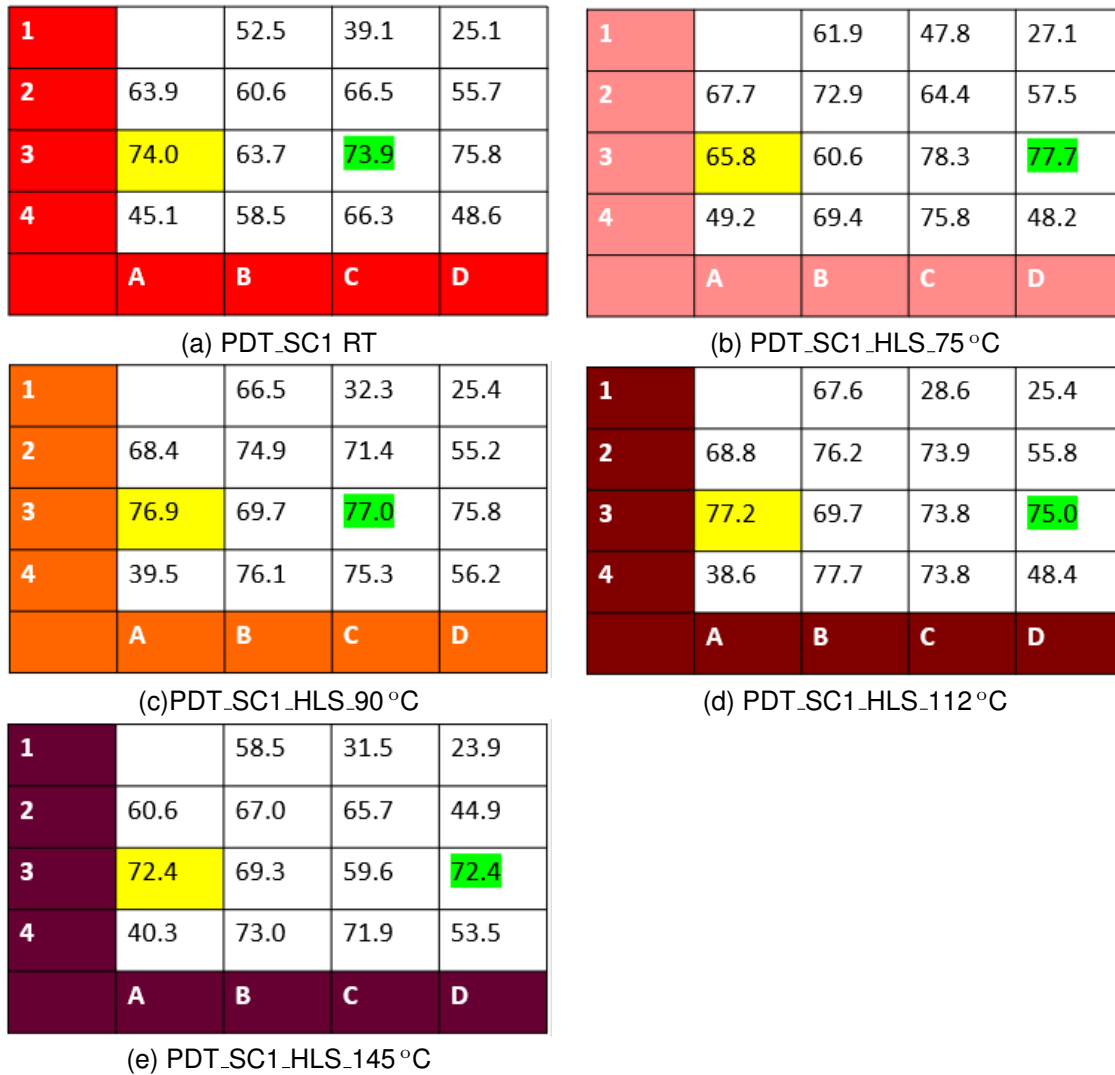
Figure 6.48: Fill Factor measurements of sample PDT_SC1 before (RT) and after Heat-Light Soaking at temperatures 75 °C, 90 °C, 112 °C and 145 °C.
