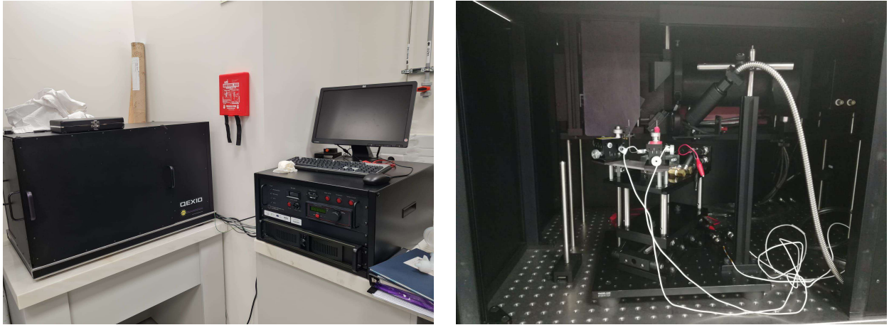
Figure 5.8: Solar Cell Quantum Efficiency Measurement System. On the left: the complete system. On the right: the black box opened. It is possible to see the platform where the cell is placed.
