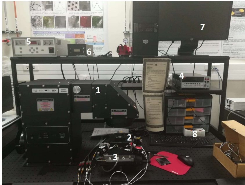
Figure 5.5: Solar simulator set-up. Legend: 1-Newport's Corporation Oriol Sol3A Class AAA Solar Simulator, Model 94043A; 2-Silicon Reference Cell; 3-Cell holder; 4-Keithley Source Meter , Model 2420; 5-Arc Lamp Power Supply, Model 69920; 6-Irradiance display; 7-Computer used for IV Test Station Software; 8-Protection Glasses 2, 6-Oriel PV Reference Cell System Model 91150V.
