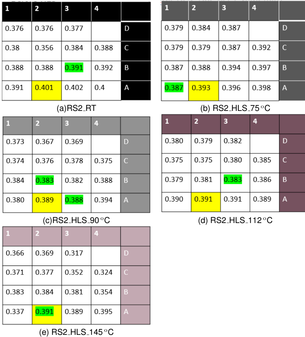
Figure 6.16: V_{OC} of the sample RS2 before (RT) and after Heat-Light Soaking at 75 °C, 90 °C, 112 °C and 145 °C.
