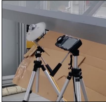
Figure 3.3 Photo of the Smp11-A pyranometer and the C-800 SpectroMaster Color Meter .
