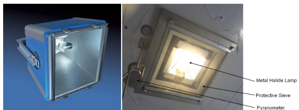
Figure 2.7 a) Floodlight SFL by Hönle , from the product catalog (Hönle, n.d.) b) Sanwood Solar Simulator for athlete training or material testing ( Sanwood , n.d.).
