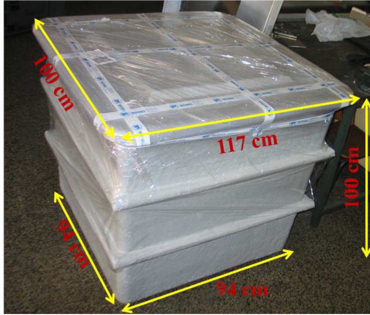
Figure 4.1: 1000 litres fiberglass container purchased by Sousa (2014) for experimental validations of the orthogonal configuration. Adapted from Sousa (2014).
