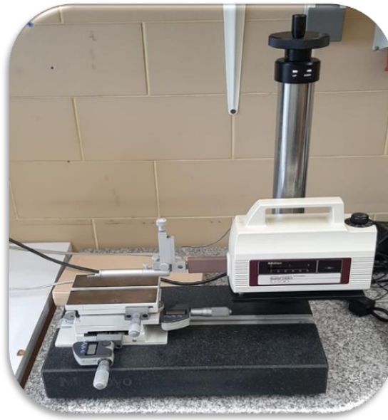
Figure 3.6. Profilometer MITUTOYO SJ-500.
