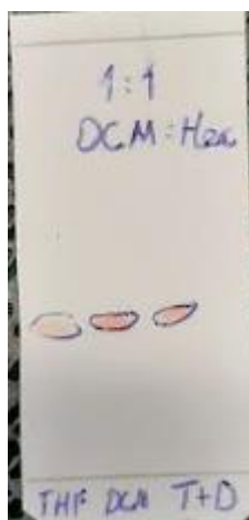
Figure 23- TLC of the dimer formed by THF, DCM and the mixture of both.
