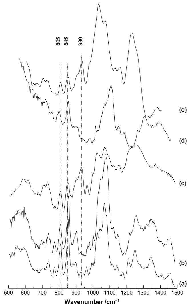
**Fig. 3.** FT-Raman (a) and FTIR-ATR (c) spectra of commercial iota-carrageenan; FTIR-ATR (d) spectra of ground seaweed sample (*Eucheuma denticulatum*); FT-Raman (b) and FTIR-ATR (e) spectra of ground seaweed sample *Calliblepharis jubata*, non-fructified thalli.
