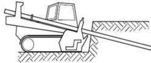
STEP 2. DRILL NAIL HOLE
