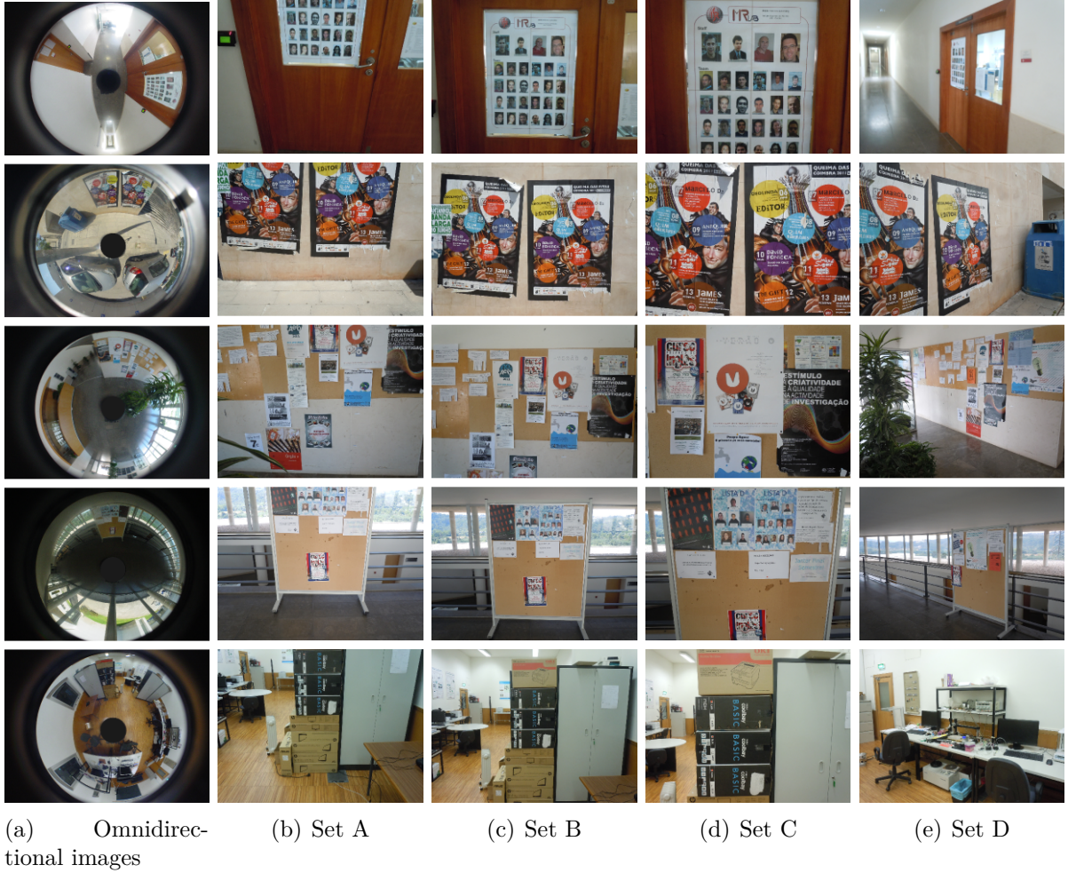
Figure 2.3: Examples of paracatadioptric images and the corresponding perspective images.
