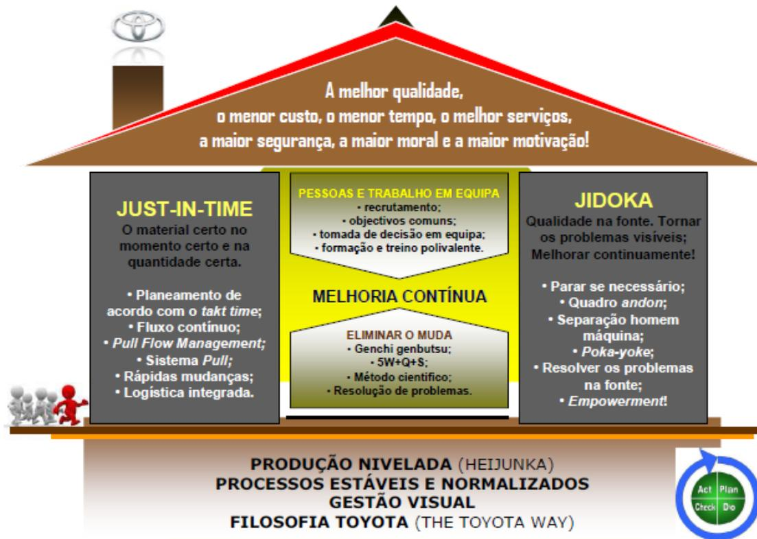
Figura 1 - A Casa da Toyota Production System (CLT, 2013)
