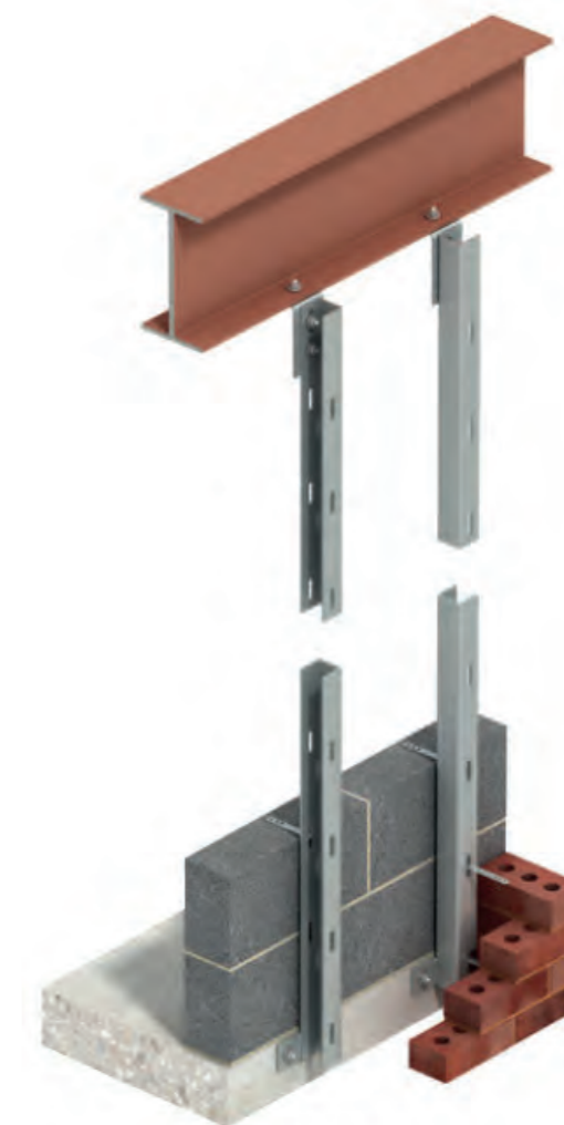
WP3 Fixed to Concrete at the Base and a Steel Beam at the Top
