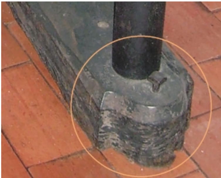
Fig. 8. Detail of the 'toe' of the T-base of the Coimbra press. Photograph by Robert Oldham.
