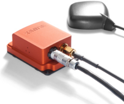
Figura B.5: Sensor Xsens MTi-G-700
