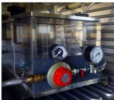
Figure 8 Customized pressure chamber inside a 37° C oven. The pressure chamber is equipped with a regulator to control the pressure.
