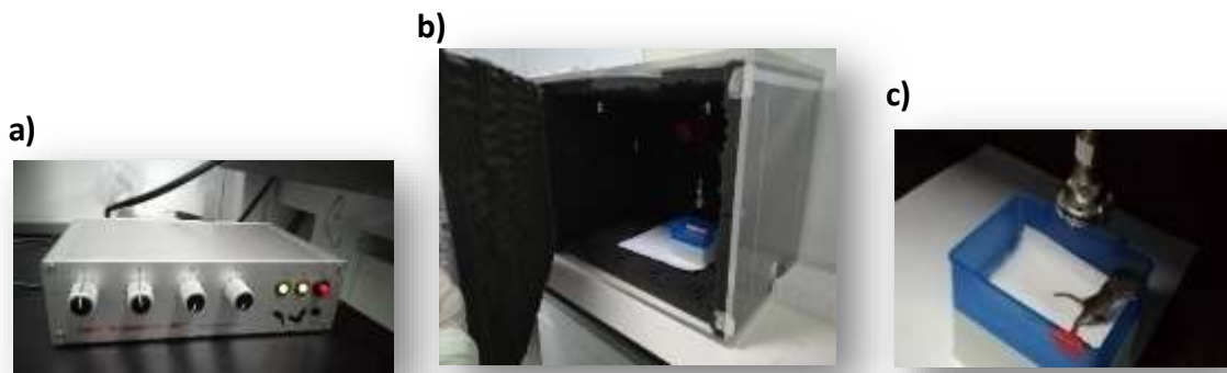
Figure 11. Ultrasonic Vocalization Recording system. Representation of the anechoic chamber used to record ultrasonic vocalizations (USVs) during behavioural tests. (a) System of regulation of the microphones' volume; (b) Anechoic chamber with acrylic sheets and covered with absorbing foam on the inside used to record vocalizations; (c) Example of a recording of a mouse pup inside the box covered in paper to control the animal's body temperature.
