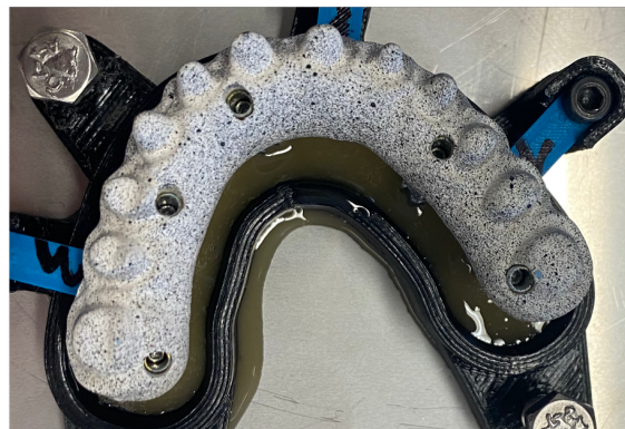
Figure 3.18: Example of speckle in a framework.
