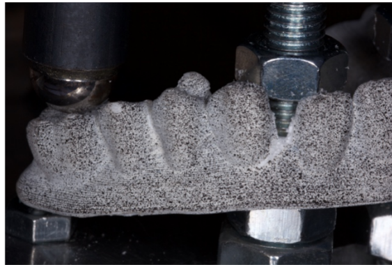
Figure 4.25: Fracture of the prosthesis made of HIPS.
