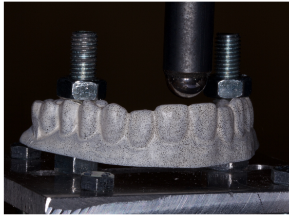
Figure 3.21: Compression of the complete prostheses in the incisors. Note the spherical surface used for the compression.
