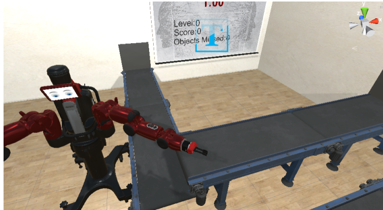
Figure 4.8: Conveyor belt that delivers the objects to Baxter.
