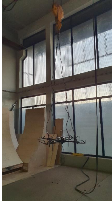
Figure 41 - Industrial crane holding drone during experimental tests
