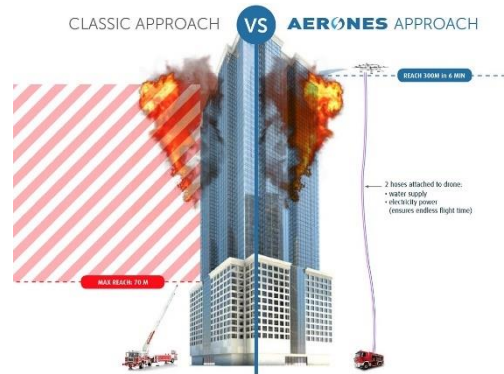
Figure 12 - Illustration of the advantage of Aeronex' drone (extracted from [10])
