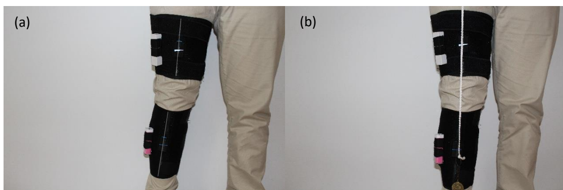
Figure 20: (a) Marks for alignment on the fabric straps, (b) pendulum align IMU instrumented knee pad
