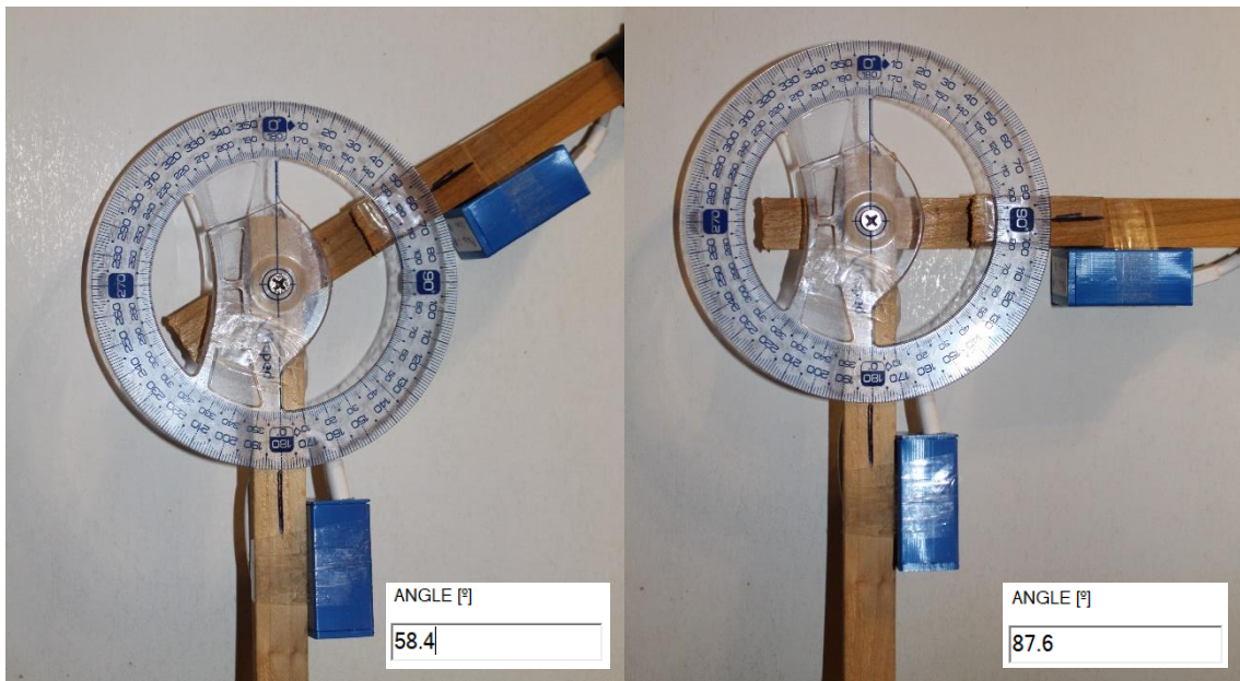
Figure 24: Verification of the IMU IKP collected values vs measured protractor values – (3) 60°, (4) 90°.
