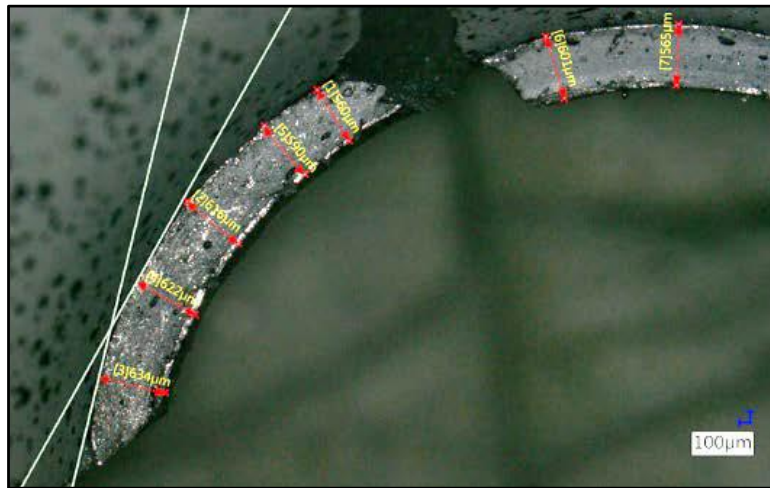
Figure 2.13. Fracture location in the hole expansion test and thickness measurement [8].
