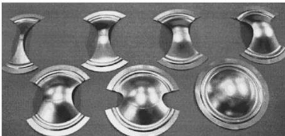
Figure 2.15. Set of specimens used in the Nakazima test for a complete FLD [2].
