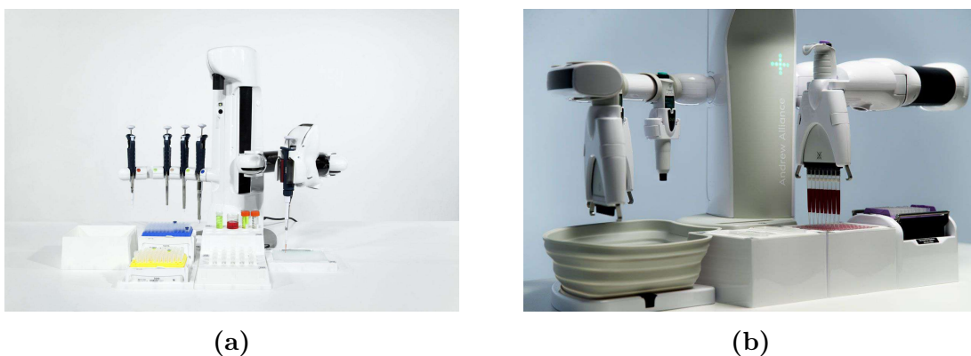
Figure 2.6: Pipetting robots from Andrew Alliance. In (a) is shown the Andrew robot [32] and in (b) is represented the Andrew+ robot [33].
