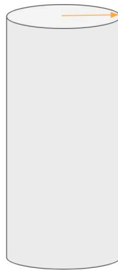
Figure 4.10. Schematic representation of the hardness analysis in the radial direction of the Co28Cr6Mo samples.
