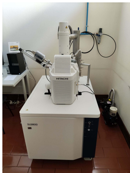
Figure 4.3. HITACHI SU3800 scanning electron microscope.
