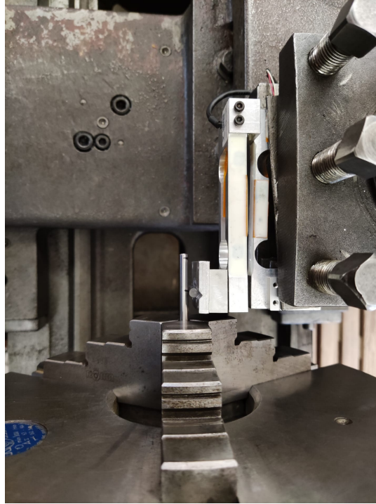
Figure 4.9. Top view of the contact between the Co28Cr6Mo and the WC cylinders. The Co28Cr6Mo cylinder is connected to the lathe, which gives it rotational and forward movement. Its sweeping area is delimited by the black marks.
