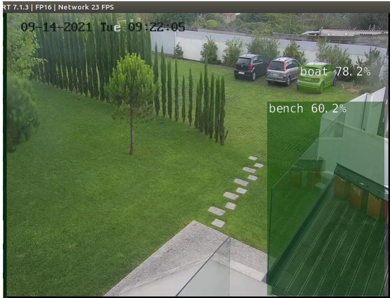
Figure 5.8: SSD-MobileNetV2 detection on Jetson.
