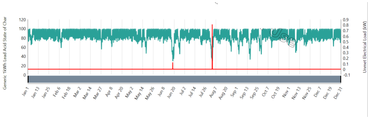
Figure 18(a): The effect of an increase in the capacity shortage of 0% on the lead-acid battery state of charge and the unmet load for the apartment building type
