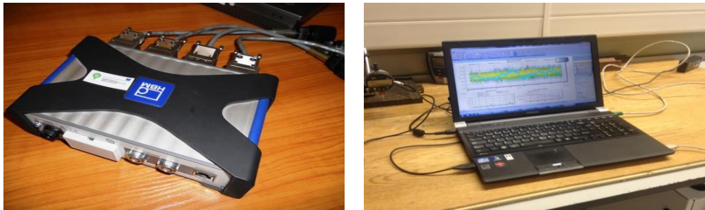
Figura 3.6 – Data Logger HBM e Software CatmanEasy V3.4.1
