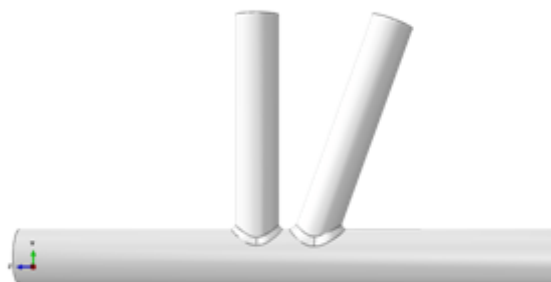
Figure 5.1- Geometry of K-joint
